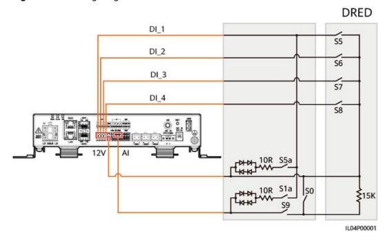
Figure 7-12 Wiring diagram for the DRM function
