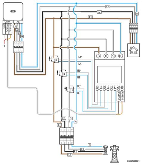
Figure 5-29 Three-phase, four-wire connection (Smart Dongle networking)
