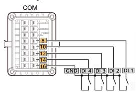
Figure 5-41 Cable connections (SmartLogger networking)
