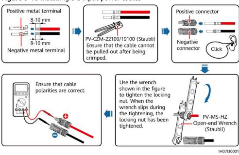
Figure 5-13 Installing DC input power cables
