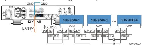
Figure 5-49 Connecting the SmartLogger to the NS protection switch
