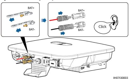
Figure 5-15 Connecting battery cables
