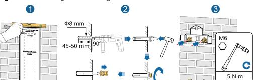
Figure 4-9 Installing the mounting bracket
