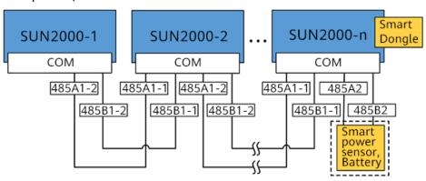
**Figure 5-21** Smart Dongle networking (the components in the dashed box are optional)
